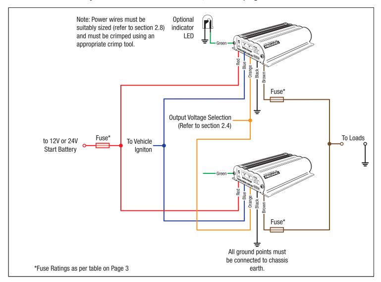
Figure 2.10.1 - Parallel Connection of two DPS units for increased output rating
