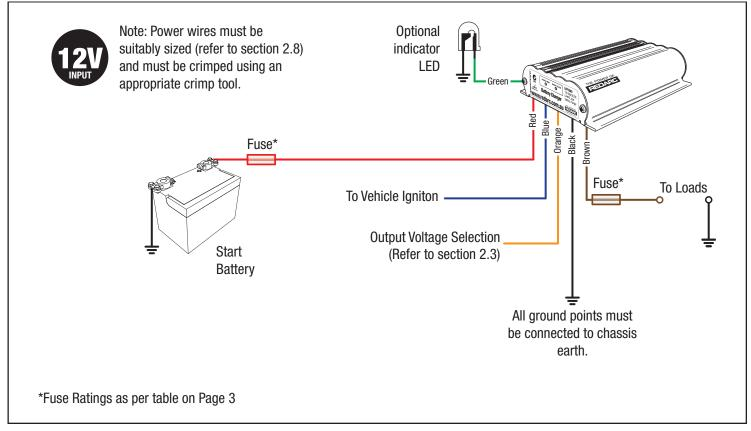
Figure 2.9.2 - Standard 12V Input setup
