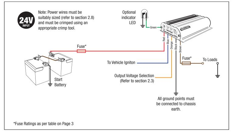
Figure 2.9.3 - Standard 24V Input setup
